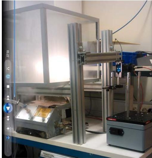
Figure 4.6: Fog chamber for validating performance of LIDAR sensor in foggy conditions
